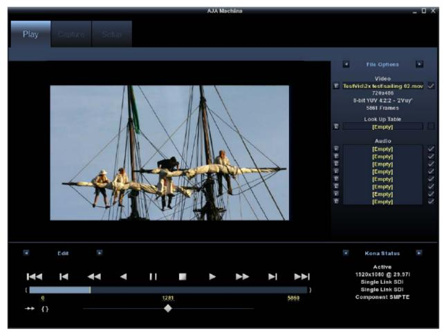
Playout controls are in Machina Play/Edit window. It is possible to play once, loop forward or loop forward-backward. Moreover, it is possible to play with variable speed. For VQL test patterns the most suitable playout mode is typically loop forward.
