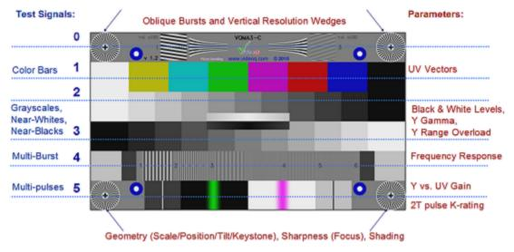
VQMA-C contains 6 relatively large bands, so it remains suitable for accurate measurements even after low bitrate coding and severe position and/or scaling errors, e.g. zoom-out down to 50% or overscan up to 105%
