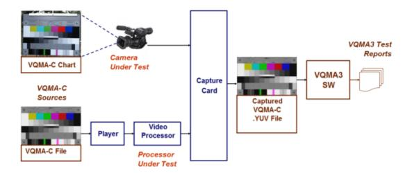
In any case the output of the device or system under the test should be routed to the VQTS-200 HDMI/DVI or SDI video input.
